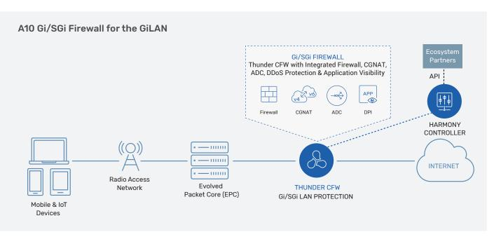
In this scenario, a mobile service provider deploys the Gi/SGi firewall to secure communication between the evolved packet core (EPC) and the internet to protect the mobile core infrastructure. Integrated carrier-grade NAT enables carriers to manage communication with both IPv4 and IPv6 address protocols. Built-in DDoS protection safeguards the NAT IP pools to avoid service interruption. Harmony Controller provides centralized management and analytics for Gi Firewall solution
