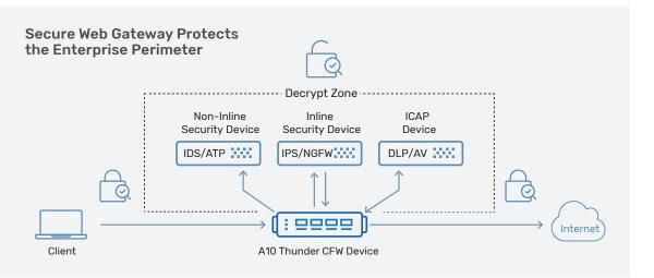
Deploy Thunder CFW, with integrated SSL Insight technology, to decrypt traffic for a variety of security products, including inline, non-inline (passive/TAP) and ICAP-enabled devices.
