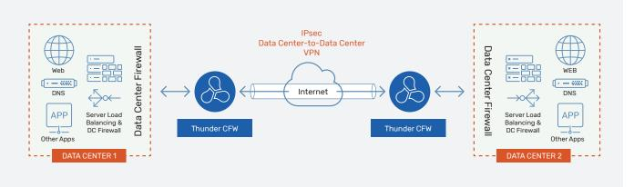
By unifying IPsec VPN, firewall and application delivery controller (ADC) capabilities, organizations are able to both load-balance traffic and protect the data center, services and related applications from DDoS attacks and other threats.
