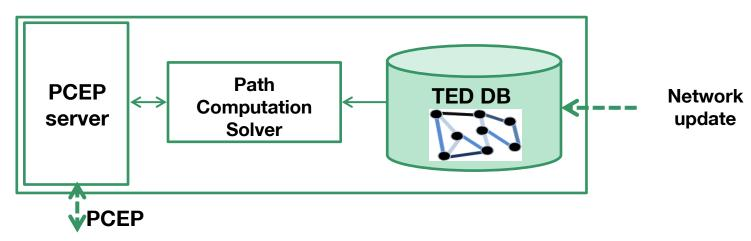
Model the network topology as a Connected Graph for performance efficiency
