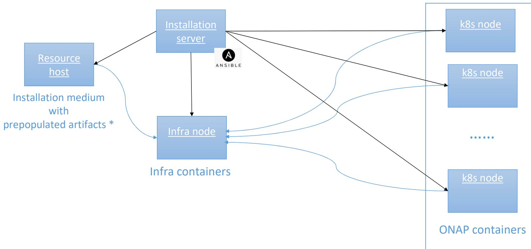
\* during installation all artifacts are copied into infra node, resource host and install server are not needed in runtime
